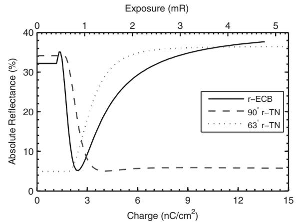
FIG. 4. Theoretical curves of the three reflective LC cell designs of interest, showing absolute reflectance as a function of charge (bottom axis) and exposure (top axis). The conversion between charge and exposure is based on a 1-mm-thick  $\alpha$ -Se layer, an x-ray spectrum of 120 kVp, 4.1 mm of added aluminum filtration, and an operating distance of 1.65 m.
