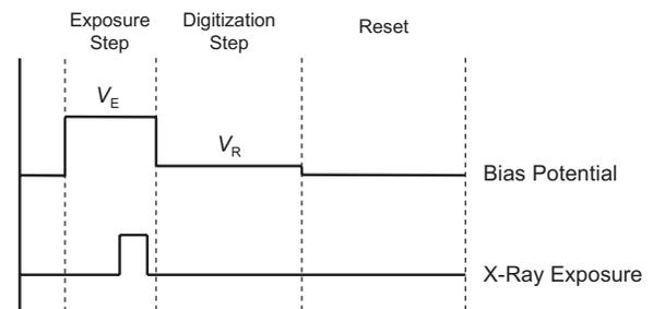
FIG. 6. Timing diagram of the operation of the XLV. During the exposure step, an exposure bias potential  $V_E$  is set to 1500 V, which corresponds to  $\sim 10 \text{ V}/\mu\text{m}$  across the *a*-Se layer. Following x-ray exposure,  $V_E$  is reduced to a readout bias potential  $V_R$  for the digitization step. Subsequently, the bias potential is removed and the image charge is erased during the reset phase.
