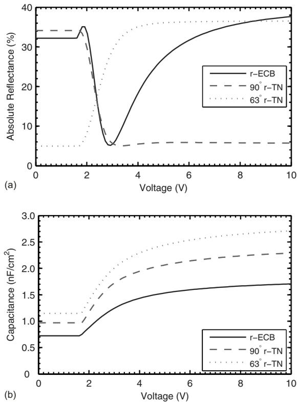
FIG. 3. Theoretical curves for the three reflective LC cell designs of interest, illustrating (a) reflectance vs applied potential and (b) capacitance vs applied potential. The parameters of the optical stacks used in the cells are summarized in Table II.
