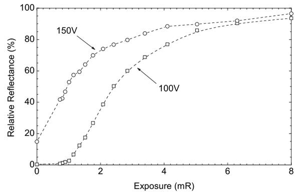
FIG. 8. Characteristic curves of the XLV prototype acquired with 100 and 150 V readout bias potential, rescaled for 1 mm  $a$ -Se thickness and 120 kVp x-ray spectrum.
