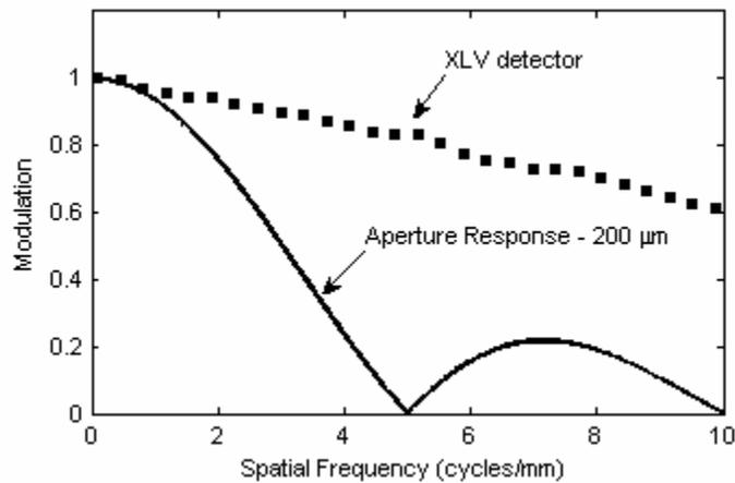
**Figure 6:** The MTF of the XLV detector (optical scanner MTF removed) and the aperture response of a 200  $\mu\text{m}$  pixel which defines the spatial resolution requirement for chest radiography. The XLV detector exceeds that of the aperture response for all spatial frequencies.
