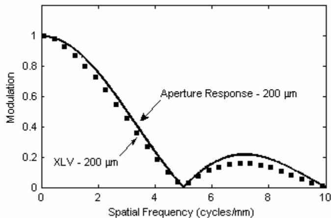
**Figure 7:** Simulated MTF of an XLV with 200  $\mu\text{m}$  pixels and the aperture response for this pixel size. The XLV follows the aperture response for all spatial frequencies indicating that for the XLV is capable of achieving the maximum resolution for this pixel size.
