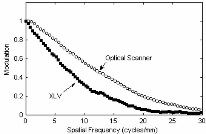
**Figure 5:** MTF of the optical scanner and entire XLV system. The MTF of the XLV was lower than that of the optical scanner for all spatial frequencies. From this graph, we can conclude that the optical scanner is the limiting factor regarding spatial resolution since the XLV MTF, which is modulated by the optical scanner MTF, was not significantly lower than that of the scanner.
