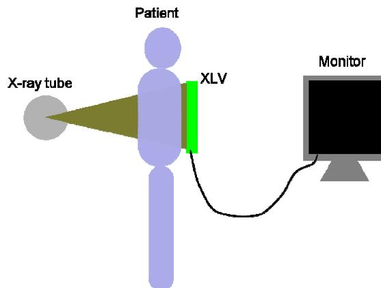
**Figure 1:** Integrated readout digital chest radiographic imaging system based on the XLV. X-rays produced in the x-ray tube are detected by an XLV detector. The image formed in the XLV detector is then digitized with an optical scanner and the image is ready for viewing at a nearby workstation.
