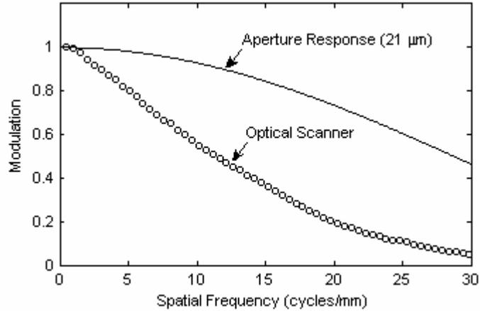
**Figure 4:** MTF of the optical scanner and aperture response for a 21  $\mu\text{m}$  pixel . The MTF of the scanner is below that of the aperture response indicating the scanner MTF was limited by the focusing optics and not the pixel size.
