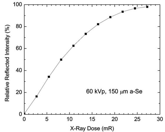
FIG. 2. XLV intensity transfer function measured experimentally. For this experiment, regions of different x-ray exposures (60 kVp spectrum) were created in a single image. To overcome the threshold voltage of the liquid-crystal cell, the XLV was uniformly exposed to radiation prior to formation of the x-ray exposure.
