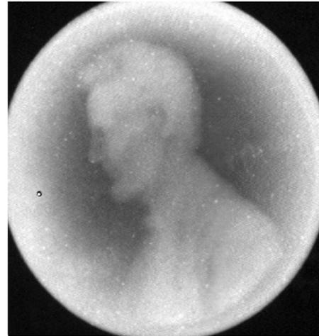
FIG. 4. Example x-ray image of a US penny taken with our prototype acquired at 60 kVp with an exposure to the coin of 27 mR.
